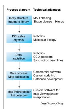
Figure 1. Process diagram for crystallographic screening showing technical advances that have improved the throughput at each step. Advances include those provided by synchrotron sources, robotics and improved computational processors.
